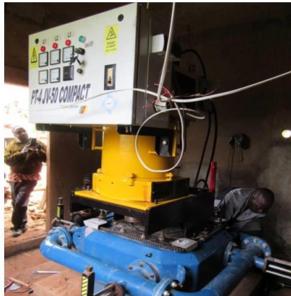
Micro-hydro powered cassava flour milling – Jakiri site
