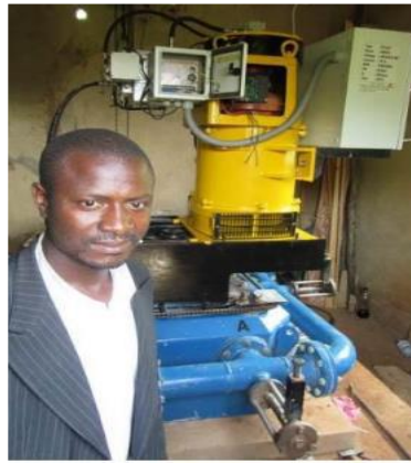
Micro-hydro powered cassava flour milling – Jakiri site
